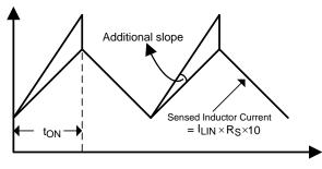
Figure 20. Slope Compensation
