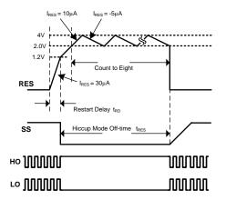
Figure 26. Hiccup Mode Overload Protection
