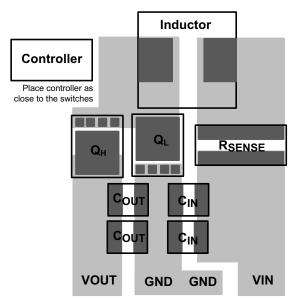
Figure 49. Power Path Layout
