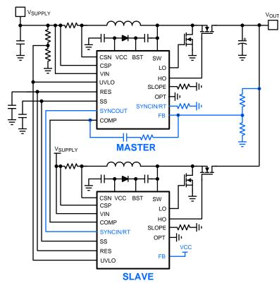
Figure 31. Dual Phase Interleaved Boost Configuration
