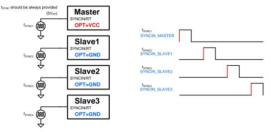
Figure 33. 4-Phase Timing Diagram Individual Clock
