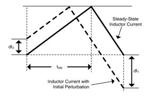
Figure 27. Effect of Initial Perturbation when  $dl_1/dl_0 < -1$
