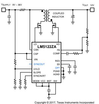
Figure 37. Sepic Converter Simplified Schematic
