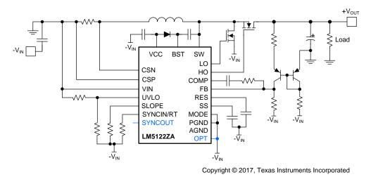
Figure 39. Negative to Positive Converter Simplified Schematic
