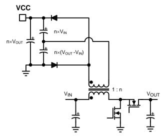
Figure 18. External Bias Supply using Transformer
