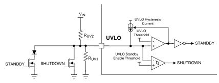
Figure 16. UVLO Remote Standby and Shutdown Control
