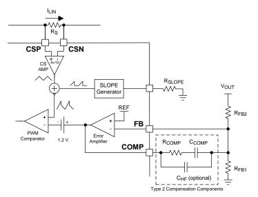
Figure 21. Feedback Configuration and PWM Comparator
