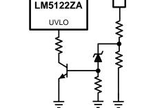
Figure 36. Output Overvoltage Protection
