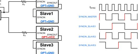
Figure 34. 4-Phase Timing Diagram Daisy Chain
